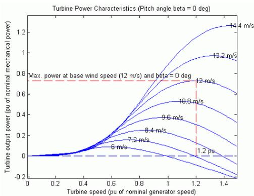
**Fig 5: Turbine Output Characteristics (Zero Pitch angle)**
