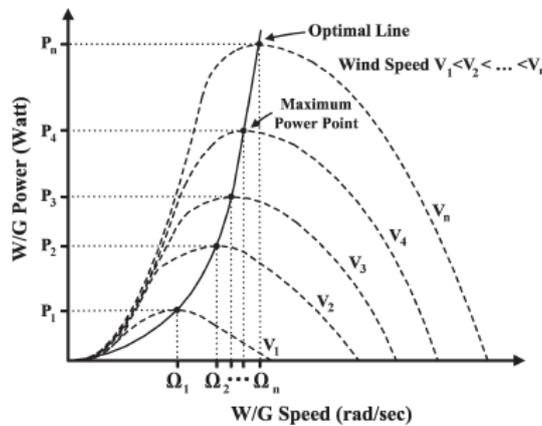
Fig 6: WG Power curves at various wind speeds
