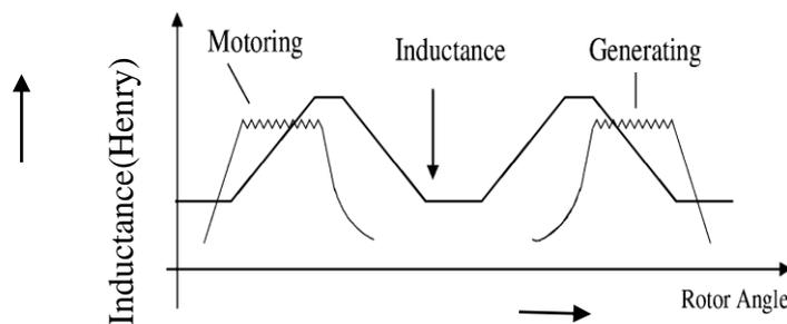
Fig 2: Inductance Vs Rotor angle
