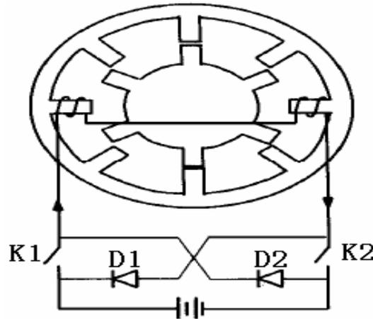
Fig 3: Cross Structure of SRG
