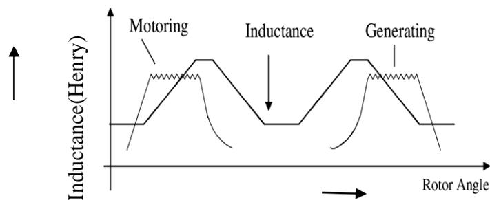
Fig 2: Inductance Vs Rotor angle
