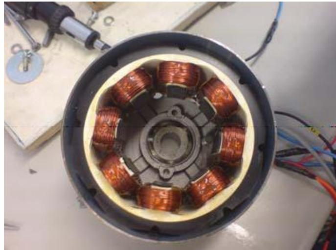
Fig 1: SRG Stator Poles and Windings
